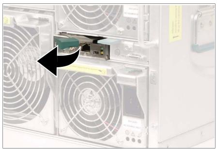
Figure 63: Disengaging the management blade
